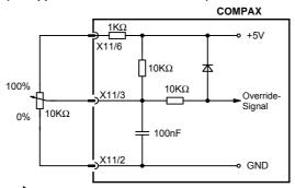
The override input is read in a cycle of 100 ms. You can continue to use the previous override connection for current applications.
